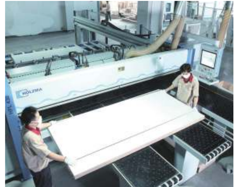
▲ German Homag Cutting Machine Computer Controlled
